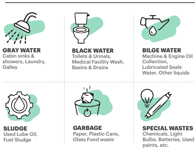
Figure 7. Waste Streams from Cruise Ships
